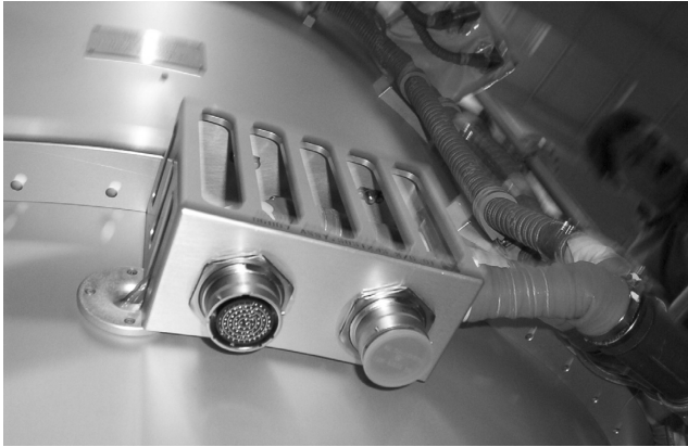
Fig. 6 Mast canister solar-array string test port connectors.
